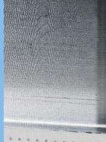
Super-fine finishing in delicate integra components, with high cutting speeds that can lead to the development of high frequencies and slight vibrations.
