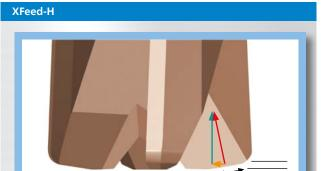
Axial force Fa stabilizes the tool and directs the cutting force in the direction of the tool holder.
