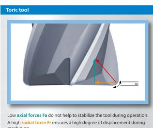
The cutting force Fc acts only on the area of the radius, meaning wear is also concentrated only on the radius. This massively increases the risk of chipping of the cutting edge.
