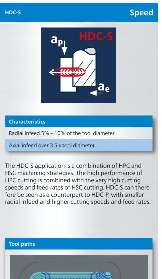
In the case of HDC-P, higher cutting forces are generated with slightly lower milling dynamics. In the case of HDC-S, the high dynamics of the machine are used for highdynamic cutting. In both applications, approximately the same metal removal rates can be achieved.
