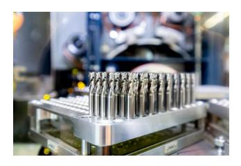
In the 2018/19 financial year, we focused on expanding our milling program for mold and die construction. With the MicroX miller program, FRAISA has created a very powerful tool portfolio that sets new standards with respect to performance, completeness and simple and fast tool selection, thereby opening up new options for the finish and superfinish machining processes in steels from 40 to 60 HRC.
