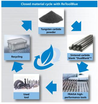
\* DualBlank = Shaft material made from high-quality recycled carbide
