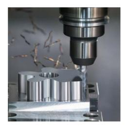
**AX-FPS** and **ToolExpert AX-FPS** for aluminum machining – maximum agility, full-slot milling up to 2xd and a penetration angle of 25°
