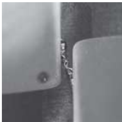
A new tool after 480 min. operating time
