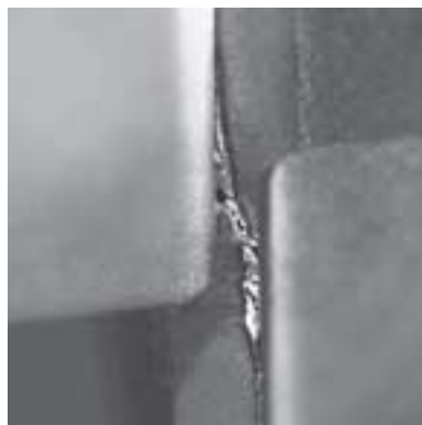
Resharpened tool (ReTool®) after 480 min. operating time
